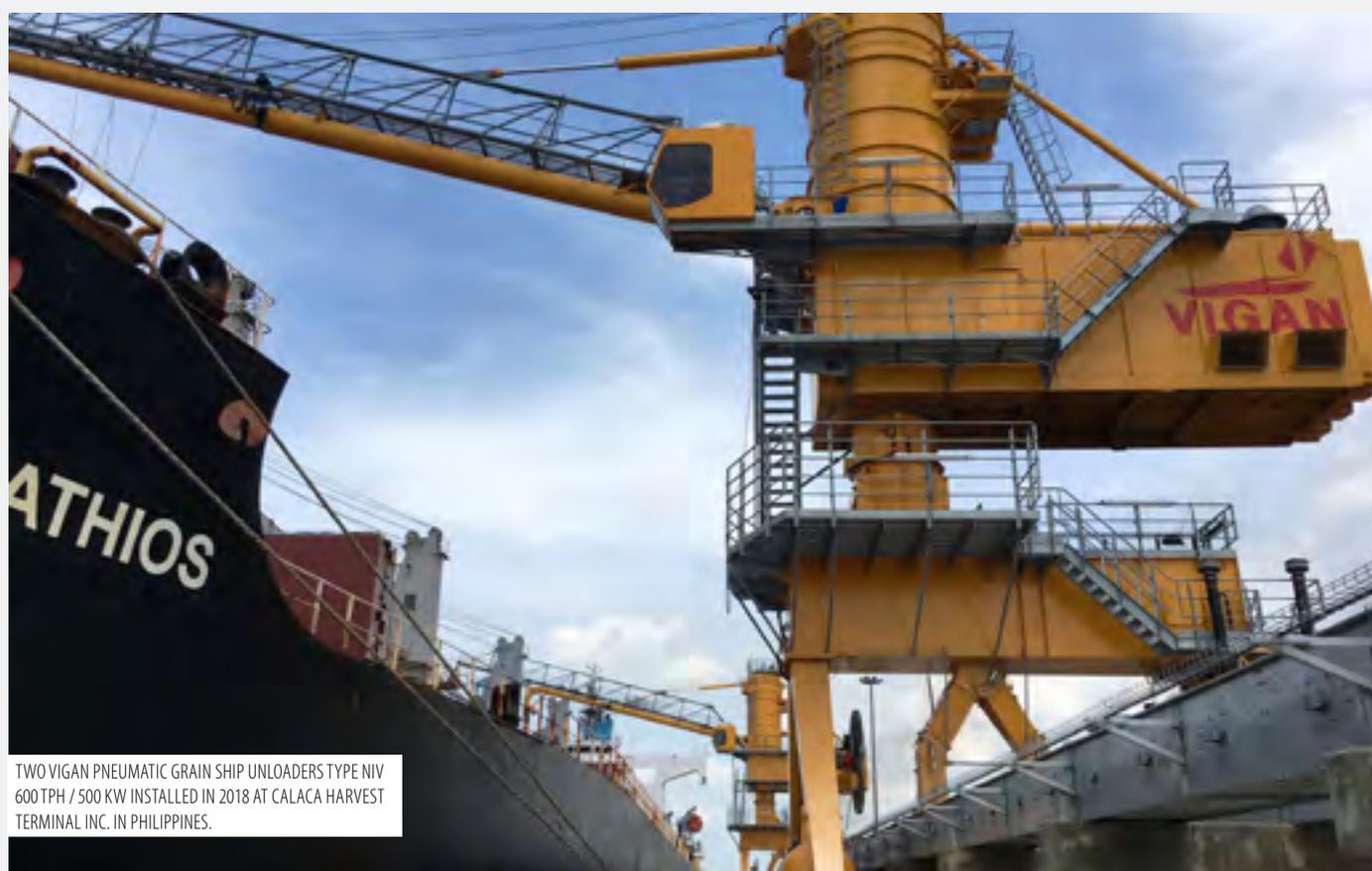
TWO VIGAN PNEUMATIC GRAIN SHIP UNLOADERS TYPE NIV 600 TPH / 500 KW INSTALLED IN 2018 AT CALACA HARVEST TERMINAL INC. IN PHILIPPINES.
