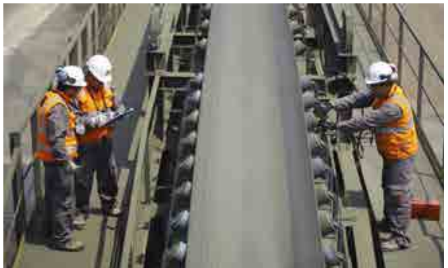
CONVEYOR SERVICE SHOULD BE PERFORMED ONLY WHEN THE BELT IS PROPERLY LOCKED, TAGGED, BLOCKED AND TESTED © MARTIN ENGINEERING 2021
