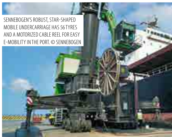
THANKS TO THE ERGONOMIALLY DESIGNED PORTCAB, THE OPERATOR CAN ENJOY A CLEAR VIEW OF THEIR WORK AREA. AS AN ADDITIONAL FEATURE, THE ZOOM CAMERA SUPPORTS THE OPERATOR WHEN LOADING THE GRAB INSIDE THE SHIP HULL, CONVENIENTLY VISIBLE ON SCREENS FROM THE OPERATOR'S SEAT © SENNEBOGEN
