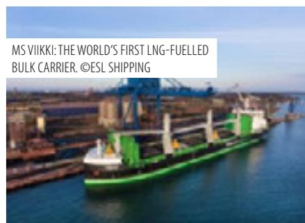
ESL Shipping is a leading Baltic carrier of dry bulk cargo operating within the sulphur emission control area. Both *Viikki* and sister ship *Haaga*, were designed in accordance with the Energy Efficiency Design Index (EEDI). LNG proved to be the most attractive fuel option, enabling the vessel design to cut CO<sub>2</sub> emissions by more than 50%, compared with traditional heavy fuel alternatives. Ice can cause rapid
