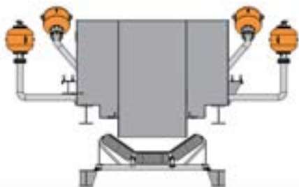
PROPER AIR CANNON PLACEMENT IN CHUTES AND SILOS CAN REDUCE ONGOING BUILD-UP
