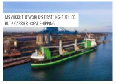
ESL Shipping is a leading Baltic carrier of dry bulk cargo operating within the sulphur emission control area. Both *Viikki* and sister ship *Haaga*, were designed in accordance with the Energy Efficiency Design Index (EEDI). LNG proved to be the most attractive fuel option, enabling the vessel design to cut CO<sup>2</sup> emissions by more than 50%, compared with traditional heavy fuel alternatives. Ice can cause rapid
