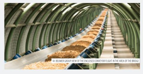
been using a 12.7km-long BEUMER Group overland conveyor to transport limestone from the quarry to the intermediate bin. The troughed belt conveyor runs through hilly terrain and over rivers and unstable ground. In 2016, BEUMER Group installed two more overland conveyors, this time with an overall length of 13.7km to transport limestone to the cement plant.
