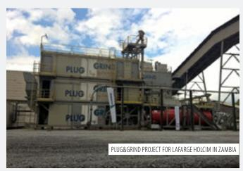
Finally, installing Plug&Grind® could see production go from 12tph to more than 70tph, depending on the market size.
