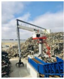
either to plug in to a shore-based power source, or alternatively operate independently using a genset.
