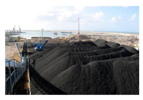
The equipment's radial boom generates a high stockpile with minimum machine movements, while its compact design allows for utilisation of irregular storage and stockpile areas.
