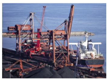
The Konecranes Gottwald Portal Harbor Crane has been installed between the two remaining gantries without stopping terminal operations
