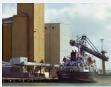
TRASMEC continuous mechanical unloader
