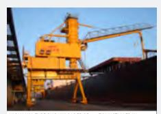
VIGAN NIV-TYPE SHIP UNLOADER OF 600 T/H INSTALLED IN TAIWAN IN 2018 AND IN THE BACKGROUND IS THE VIGAN NIV 600 T/H INSTALLED IN 2014
