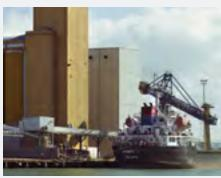
TRANSMEC continuous mechanical unloader
