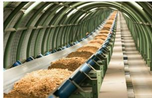
A second project will now include two additional overland conveyors, with an overall length of 13.7km, transporting limestone to the cement plant. Unlike the first project, the task here was to build the conveyor across inhabited areas. Noise emission limitations set forth by the government also needed to be considered.
