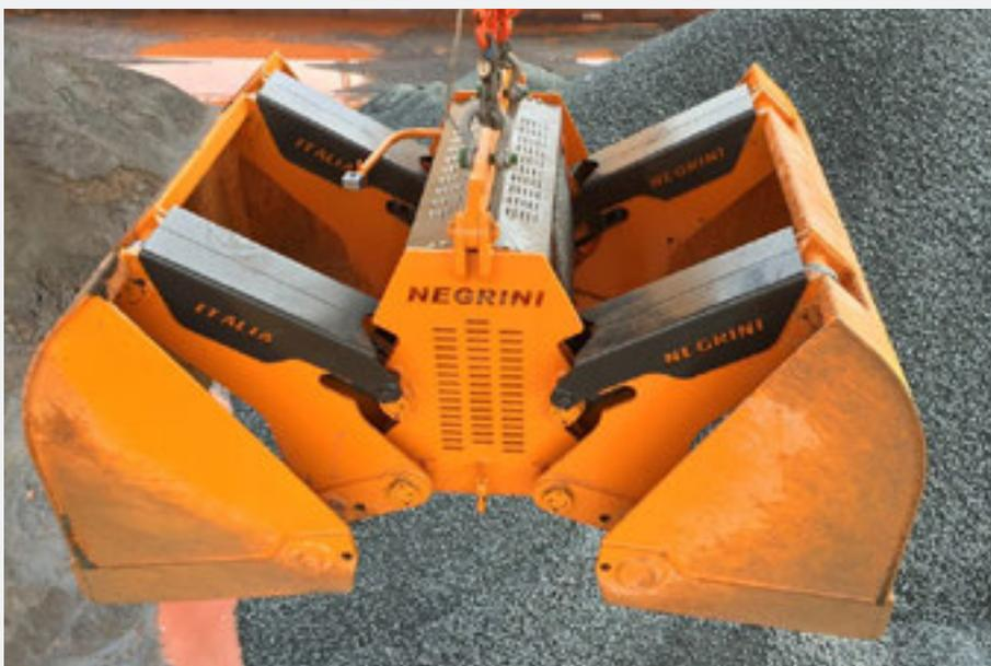
protected by two commercial "o-ring" type gaskets. These are blocked in place and do not allow any dirt to enter. The pressure on the outside allows the grease to be released, thereby lubricating the walls and removing dirt.
