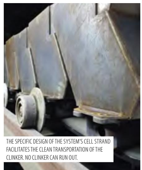
THE SPECIFIC DESIGN OF THE SYSTEM'S CELL STRAND FACILITATES THE CLEAN TRANSPORTATION OF THE CLINKER. NO CLINKER CAN RUN OUT.
