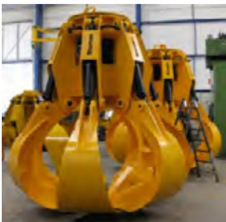
Should the product be heavy or compacted, of big granulation or sometimes mixed with light products or plastic packages, the grab works at a lower or higher speed, regulating the penetration force required and with the adequate dragging of the material. It changes the speed and regulates the pressure according to the material characteristics in each moment, the company says.
