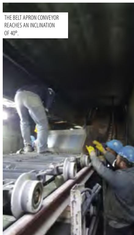
THE BELT APRON CONVEYOR REACHES AN INCLINATION OF 40°.
