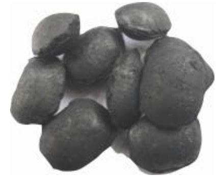
Roller Briquetted 12 - 50mm
